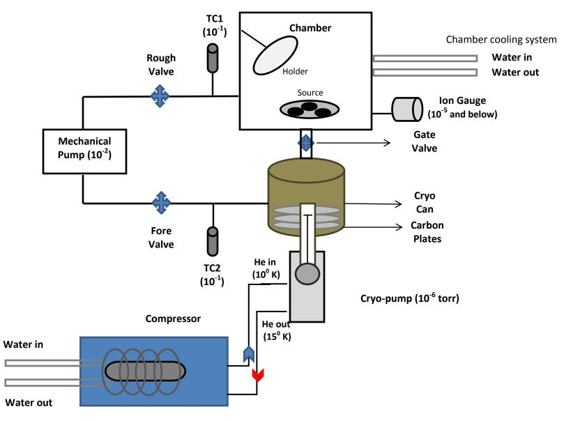
Cryo-pump cooling system
